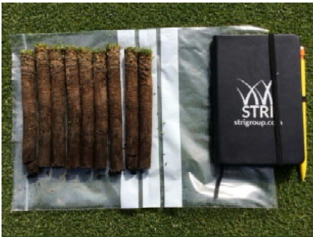
Figure 3: Soil samples collected on the greens revealed the extent of sand integration but a higher than desirable thatch accumulation remains in the top 50mm of the profile.
